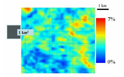
**Figure 3.** Fast velocity – slow velocity time slice, Rocky Mountains showing channel with high anisotropy embedded in shales and mudstones with low anisotropy.
